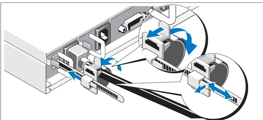
Release the latch on the retainer unit and pull the clamping ring towards the end of the strip. Open the clamping ring and insert the power cable. Close and push back the clamping ring until it is as close as possible to the system. Check to ensure that the power cable is secured to the system.
